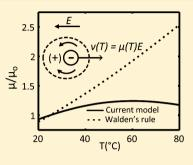
Effects on ElectroPhoresis (STEEP). We validated our model using conductivity and pH measurements across a temperature variation of 25-70 °C for a set of electrolytes routinely used in electrophoresis. The model accurately captures electrolyte solution pH and conductivity, including important effects not captured by simple Walden-type relations.
